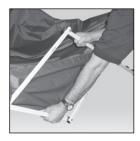
**4.** Grasp the top and bottom of diamond-shaped area of trusses by "open" sticker. Slightly lift shelter up and push hands together while stepping backwards until shelter is fully opened. **Be careful not to pinch fingers.**
