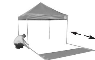
1. Position legs perpendicular to those of the Instant Shelter® where the sliders were installed.
