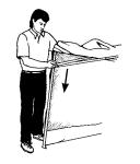
2. Release auto-slider at all three corners by slightly lifting up on slider with one hand while depressing snap button with other hand. Once snap button is depressed, push slider down past snap button.
