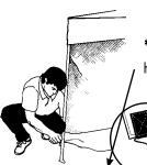
\*3. Attach J-hooks sewn on the top into holes located in the bottom of the legs.
