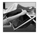
**3.** Grasp top and bottom of diamond-shaped area of trusses by "close" sticker and slightly lift up. Shake shelter slightly, pulling hands apart, until you are able to close shelter with your hands completely.
