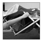
4. Grasp the top and bottom of diamond-shaped area of trusses by "open" sticker. Slightly lift shelter up and push hands together while stepping backwards until shelter is fully opened. Be careful not to pinch fingers or pull backwards too hard.
