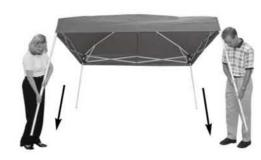
4. With partner, lift two adjacent outer legs up and slide out the inner legs until the snap button locks. Repeat on the opposite legs - make sure to do two legs at a time on same side.
