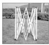
Place your QUEST™ frame in the center of area to be shaded. With partner on opposite side, grasp outer legs, lift off the ground, and step backwards - stopping at full arms' length, approximate size as shown above.
