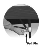
3. Release Pull Pin at each corner by first lifting valance fabric away from slider. With one hand push up on truss near the Pull Pin, pull the pin out to release. NOTE: It is much easier to release Pull Pin when the shelter weight has been removed from the Pull Pin.
