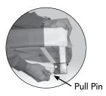
**2.** Release pull pin at each corner by first lifting valance fabric away from slider. With one hand hold the top of the leg while pulling the pin out to release.
