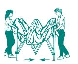
6. Grasp adjacent outer legs and push shelter together until fully closed. Be careful not to pinch fingers! Do not push hard. Put cover bag over shelter.
