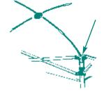
**5b.** Firmly insert end of flex rod that is attached to frame in plastic corner bracket holes. Upon insertion, all four rods should point at each other.
