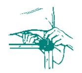
4. Release auto slider at all four corners by slightly lifting up on slider with one hand while depressing snap button with other hand. Once snap button is depressed, push slider down past snap button.
