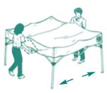
2. Grasp the top and bottom of diamondshaped area of trusses. Slightly lift shelter up and push hands together while stepping backwards until shelter is fully opened.
