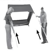
**2.** Disengage the Auto Slider® at each corner. With one hand pull down on the truss near the slider and depress the snap button. Repeat on all corners.
