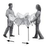
**4.** Grasp the bottom of the diamond shaped area of trusses on opposite sides. Lift up and step backwards until shelter is fully opened, **being careful not to pinch fingers.**
