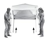
1. With a partner, slightly lift up two adjacent outer legs, depress snap button and telescope inner legs into outer legs. Repeat on the opposite legs - making sure to do two legs at a time.
