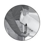
**5.** To engage the slider at each corner, first lift the fabric top off of the slider, then with one hand hold the top of the leg while pushing up on the slider with the other hand. The pull pin will engage the hole. Pull down the fabric top over the slider. Repeat on remaining three corners.
