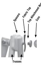
\***7.** Unscrew top attachment nut from bolt. Place grommeted fabric top over the bolt, screw on top attachment nut and tighten until snug. **Top should rotate easily - do not overtighten.** Repeat this procedure on the remaining grommets.
