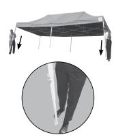
two outer legs as shown 1" and lower the inner legs until toggle button locks. Repeat on middle leg on same side. Repeat on opposite legs.
