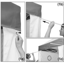
**Step 1.** (1a)Locate the awning slot hole, just below the top valance, on the front of the shelter. (1b) Insert awning pole through the sidewall wrap fabric hole and into slider awning bracket. (1c) Repeat on opposite side.
