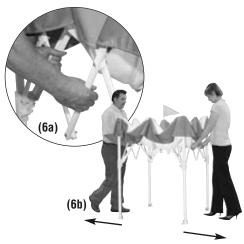
**Step 6.** (6a) Grasp the bottom of the diamond shaped area of trusses on opposite sides. (6b) Lift up off the ground and step backwards until shelter is fully opened, being careful not to pinch fingers.
