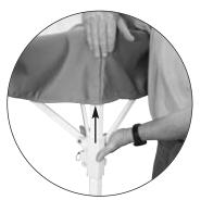
**Step 7.** To engage the slider at each corner, slightly lift the fabric top off the slider, then with one hand hold the top of the leg while pushing up on the slider with the other hand. The pull pin will engage into the outer leg pull pin hole. Pull down the fabric top back over the slider. Repeat on remaining three corners.
