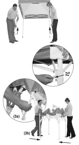
**Step 1.** With a partner, slightly lift up two adjacent outer legs, depress toggle levers and telescope inner legs into outer legs. Repeat on the opposite legs, making sure to do two legs at a time.
