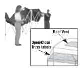
\*2. Unfold the fabric top ensuring the roof vents in the top are located on the adjacent side to the Open/Close truss labels.
