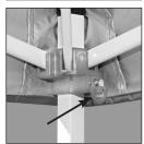
**5.** Engage the Pull Pin Auto Slider® at each corner by pushing up on slider with one hand while pushing down on top of leg with other hand. The pull pin will engage in hole. Repeat step on remaining legs.
